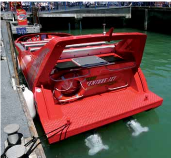
BELOW: The blunt end with the protective platform and raised hatch. Note the missing life ring
