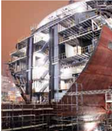
The keel laying or in this case the first section
