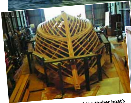
ABOVE: The heart of the timber boat's frames and stringers seen during construction
