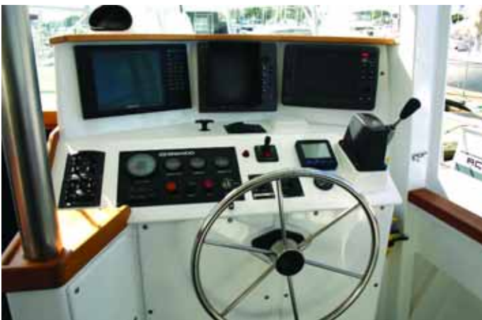
The helmstation, while compact, provides easy access to all navigational aids and controls, with good vision forward
