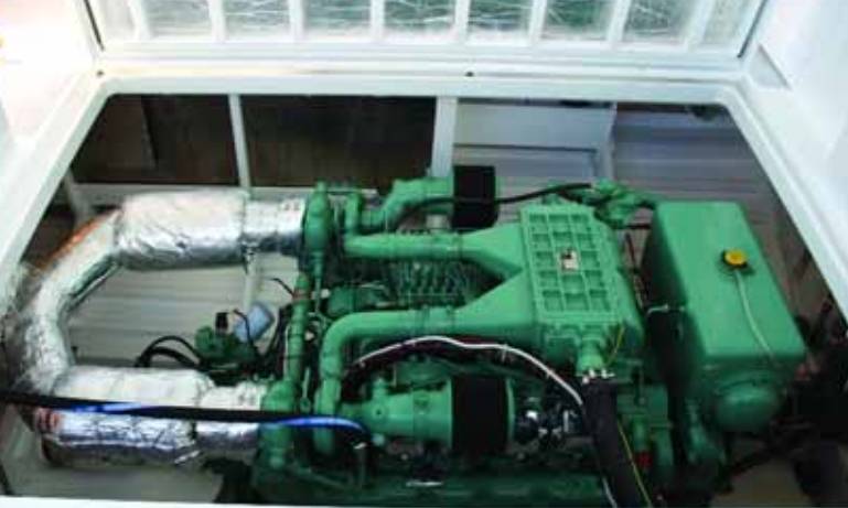
The large Daewoo engine may be accessed from below or by lifting the deck service hatch
