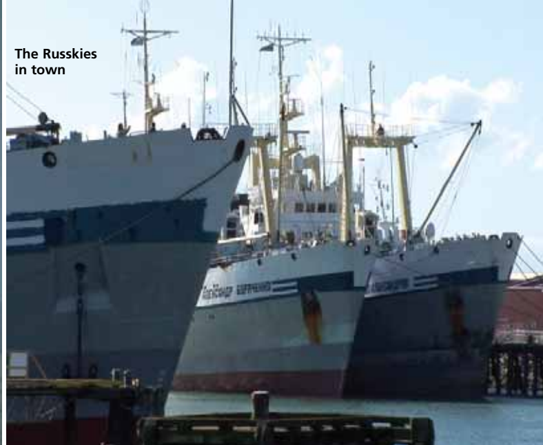
Ships like this can catch and pack 1500 to 2000 tonnes of frozen fish per trip
