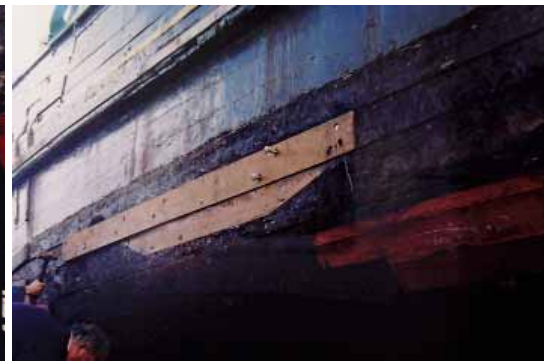
The hole filled with new planks of macrocarpa
