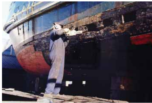
Giving the toredia a hell of a fright as I cut into the 10in x 3in kauri planking
