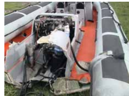
When the RHIB was ripped out of her secure cradle and davits, the transom and jet unit was left hanging in the ship
