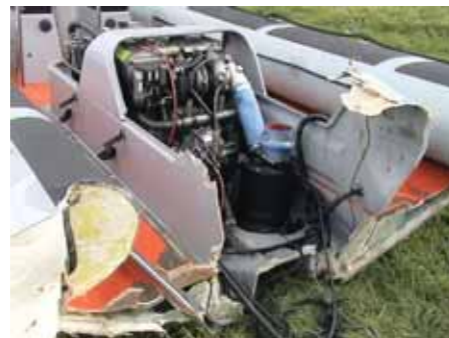
When the RHIB was ripped out of her secure cradle and davits, the transom and jet unit was left hanging in the ship
